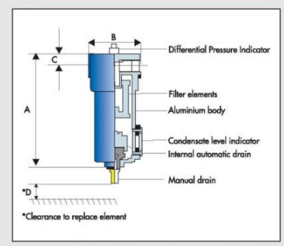
Accessories • Differential Pressure Gauge • Automatic Drain Valve
