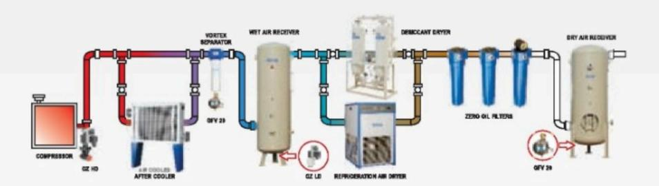
This comprehensive range of high efficiency coalescing filters will remove oil, dirt, odour and water from the compressed air supply, therefore offering complete protection to all equipment installed downstream.
